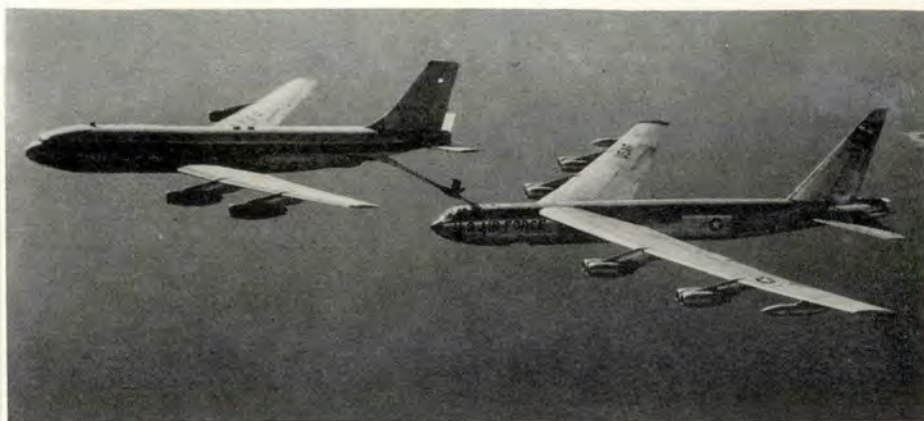
For high-speed, inflight refueling the KC-135 carries a special boom.
