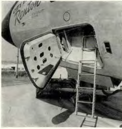
Above, both entry and escape exit is shown. The door swings out to provide wind screen.
