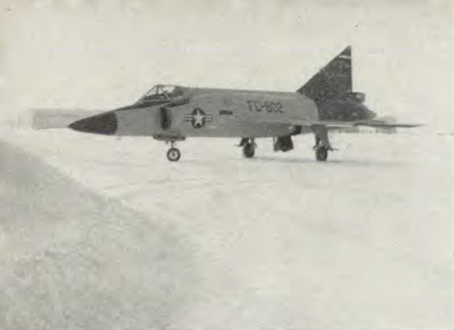
Use brakes and power with care when taxiing. Lined up with full power, brakes won't hold.
