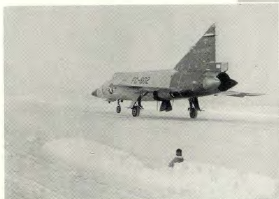
Use brakes and power with care when taxiing. Lined up with full power, brakes won't hold.
